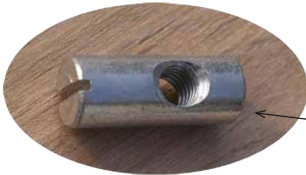
**NOTE:** all the holes for the “barrel nuts” are on the same side. This helps prevent having a part upside down or backwards (there are 8 barrel nuts per side). Their location is noted below.
