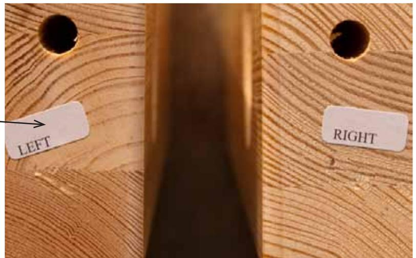
D. Assemble either right or left side first, then repeat for the other side. Attach, as the first step, the *knee beam member* to the *mid-upright* using 2 dowels and long bolt, washer and barrel nut. Then add the *cloth beam upright* to this using 2 dowels (#2 on the factory copy). Note that the cloth beam hole in the cloth beam upright centers on the notch. These first few assemblies are noted in blue text below and circled with an indication of the order of assembly.
