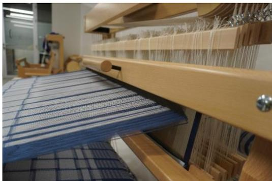
When the treadle is pressed, the lower half of the shed is on the shuttle race.
