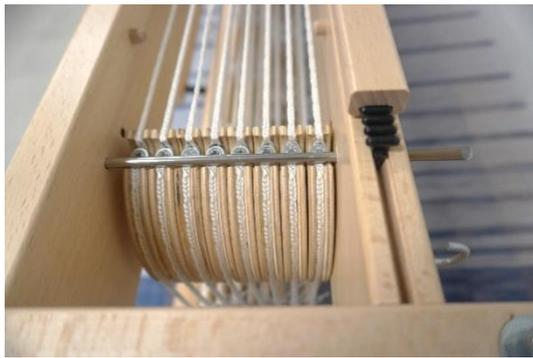
Use the blocking pin to block the cam while threading and tying up treadles. The shafts and lams are all at the same height.
