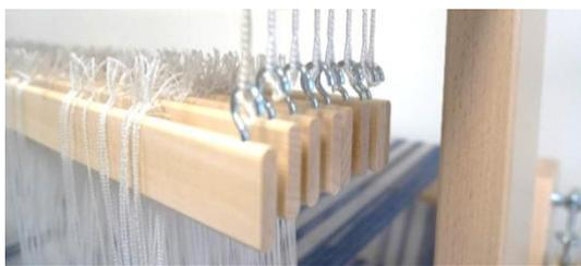
The shafts are attached to the shaft and lam cords with hooks. All hooks must be screwed in to the same depth.
