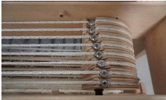
**Cam** – after adjustment, cam 1 for shaft 1, is turned more to the right than cam 8 (shaft 8).
